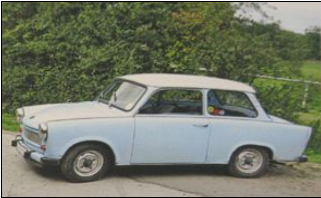
A late model Trabant with 600cc two-stroke engine
